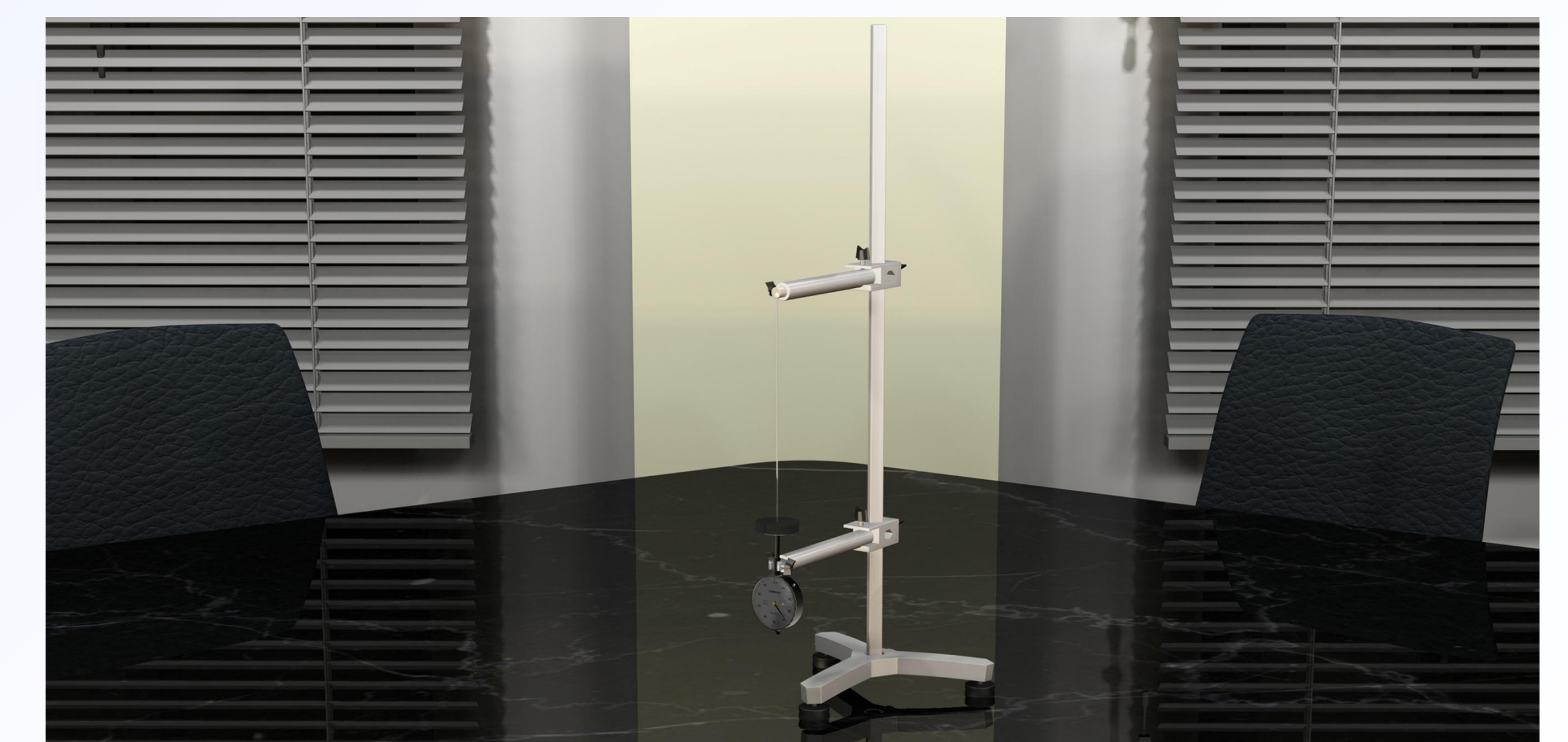
Figure 2 A simple Young's modulus apparatus
