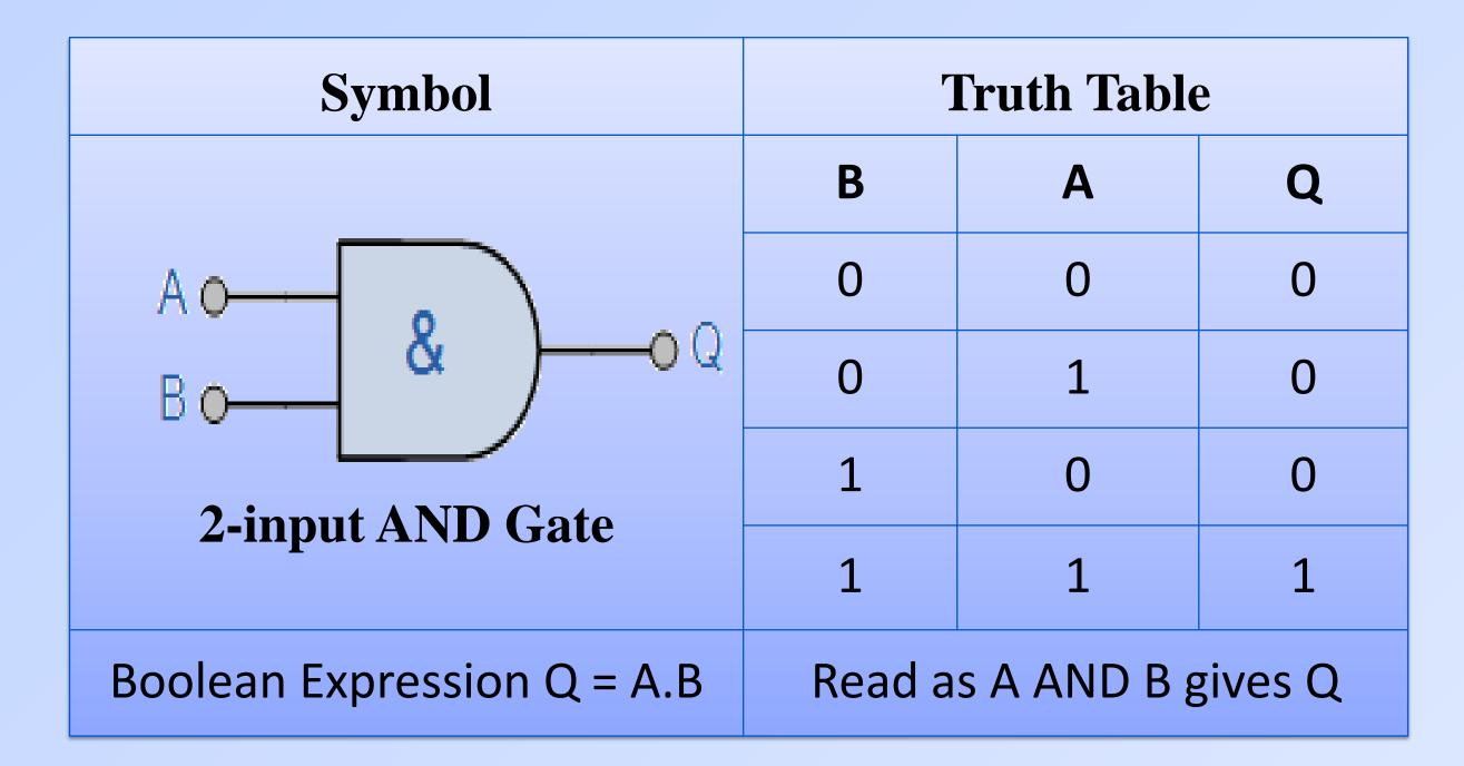
Figure 1. Logic symbols and truth table for the AND function
